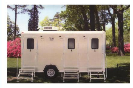
The 18' Economy Mobile Restroom trailers are perfect for those situations where elegance is a must but where space is limited. These units features fresh hot and cold running water, metering faucets, stereo sound system, heating and air conditioning, interior and exterior lighting, oak vanity cabinets, porcelain toilets and sinks, and separate entrance doors for both the women and men areas.
